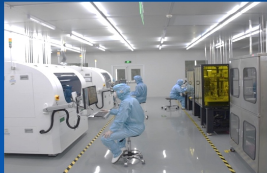
Die Bond and Test Stations for producing POET-designed Optical Engines
