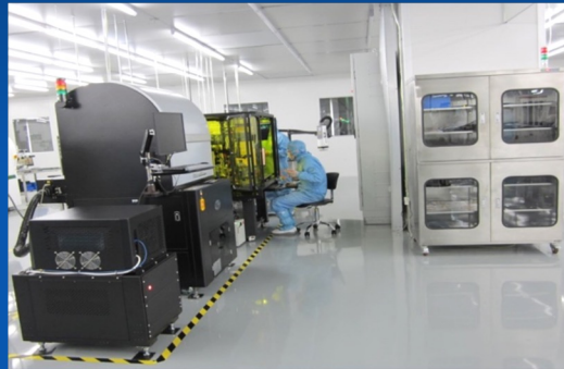
Die Bond and Test Stations for producing POET-designed Optical Engines
