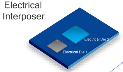
Typical electrical interposer with high-speed electrical connections among devices has been commonly used in devices like cell phones
